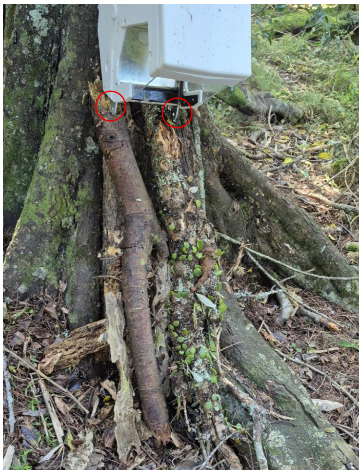
Figure 3: Example of a natural ramp to encourage rat and stoat interactions on a raised trap deployment. A ramp can also be fitted to the base of the trap, using the holes provided (circled in red in image).
