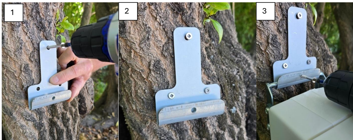
Figure 2: Attaching a bracket prior and CSL Multi-trap to tree or post.
