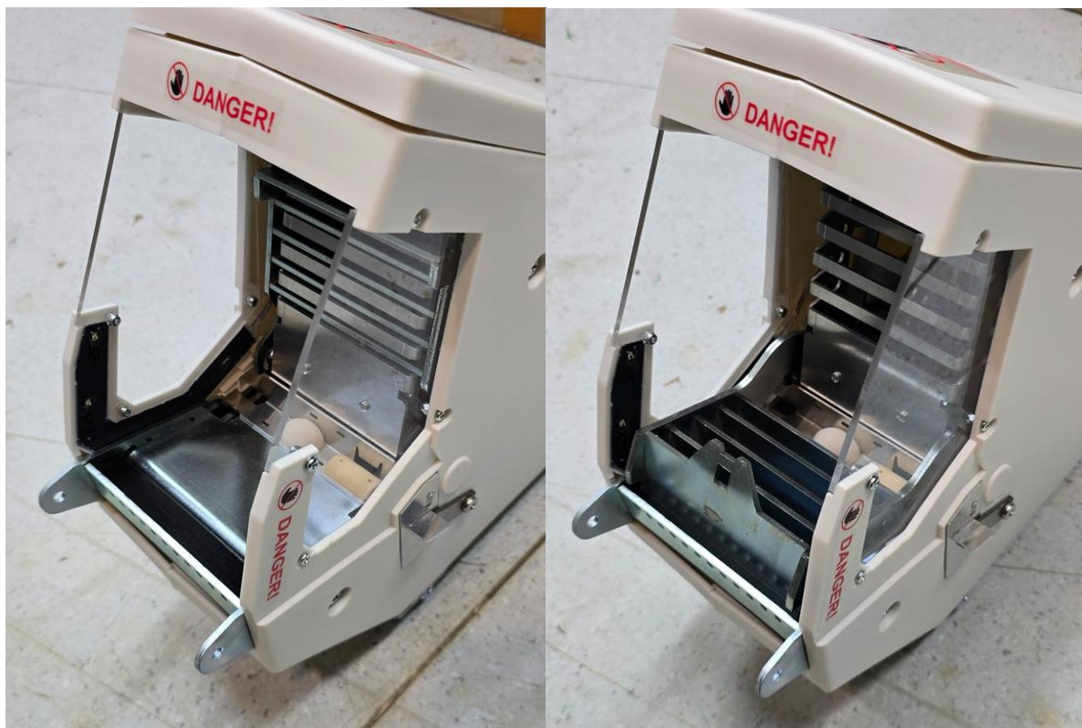
Figure 9: Kill bar positioning in the Multi-trap 1) kill bar is up and trap is set, and 2) kill bar is disarmed and safe to handle.
